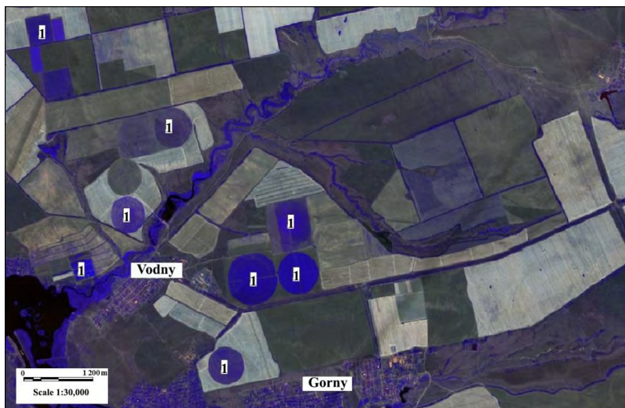
Fig. 7. Irrigated areas (1) on a Sentinel-2 image obtained on 27/07/2020, channels 2, 3 and 4 (green, red and near infrared; Gorokhova et al., 2021).
